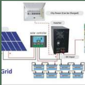
Off Grid Solar Power with battery bank
